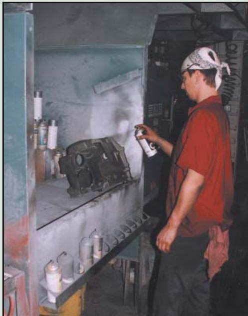
**Before reassembly, many components receive a fresh coat of paint.**
