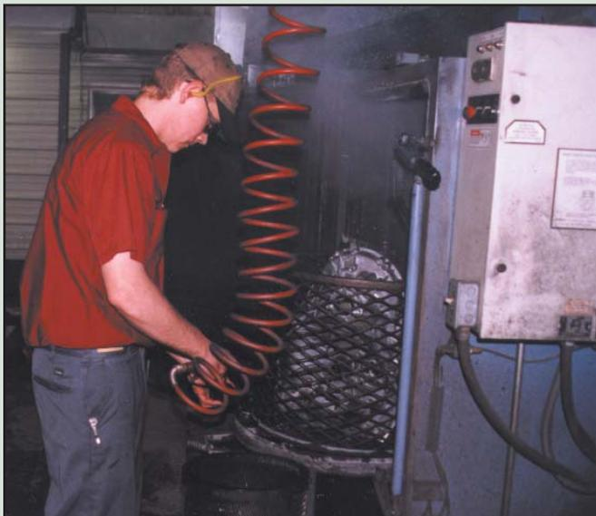
**Loading a disassembled unit into the parts washer.**
