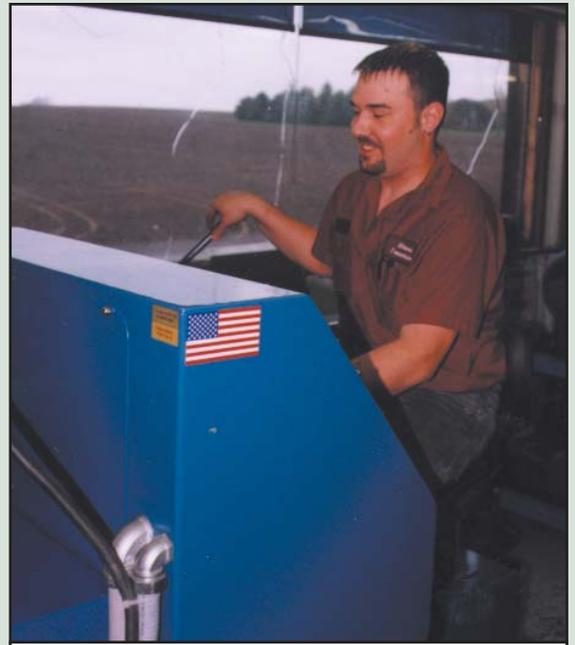
**Designed by founder Ray Schoenfelder and made to his specifications by Axi-Line, two dynamometers allow transmission testers to sit in a cockpit and control the transmission while observing the test parameters.**
