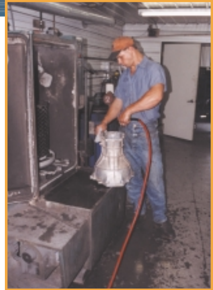
Whether a core is to be rebuilt or harvested for parts, the first step is a thorough cleaning (Jeff Schoenfelder).
