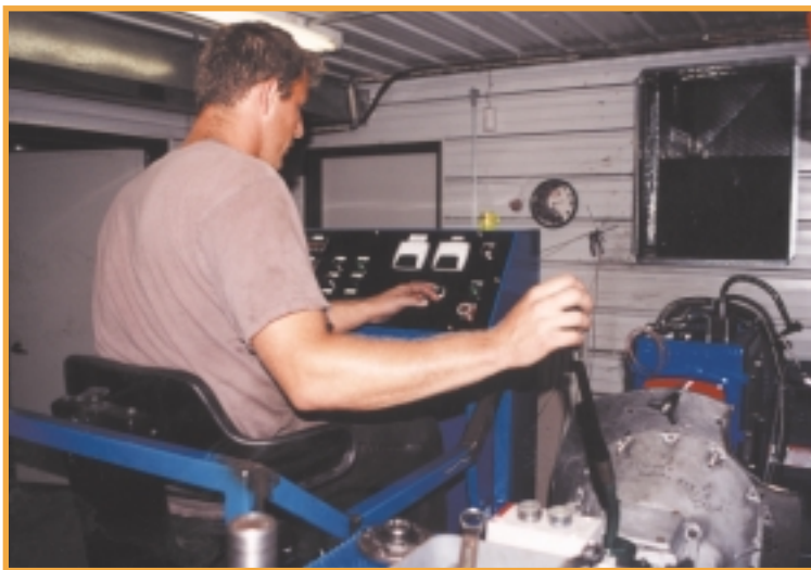
An extensively customized Axi-Line dynamometer allows the operator, Tom Stofferahan, to sit in a simulated cab, simultaneously shifting the transmission and monitoring the analytic read-outs.
